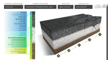
distress, road type, and the surface type. In the top photo, an urban local asphalt road in good condition, with some longitudinal and transverse cracks is a candidate for fog seal, slurry seal, microsurfacing, ultra-thin lift, chip seal, and others. Take a moment to experiment with the tool and you will see that it is an easy way to narrow down your
